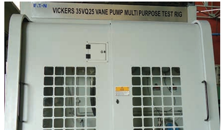
Figure 7. Eaton-Vickers 35VQ25 pump test stand made at Eaton India facility.
