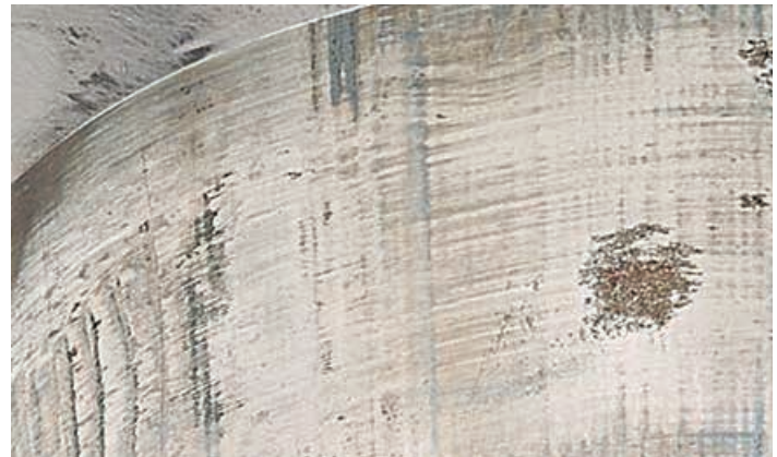
Figure 5. A cam ring of a vane pump was damaged due to lack of anti-wear properties.
