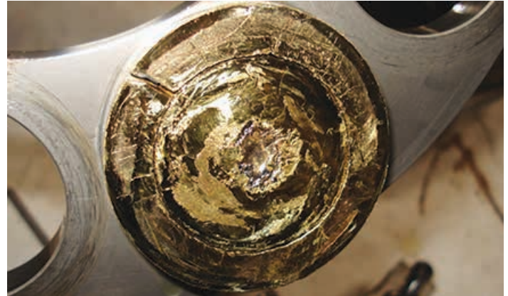
Figure 10. Contamination, lack of lubrication, and material incompatibility contributed to the failure of this piston shoe.
