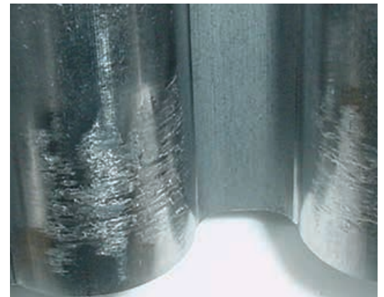
Figure 1. Low viscosity can allow metal-to-metal contact and lead to damaged components.
