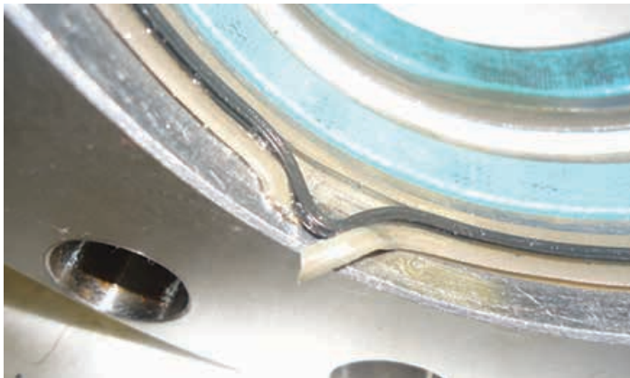
Figure 9. Rubber gasket extruded due to excess elongation caused by incompatible fluid.
