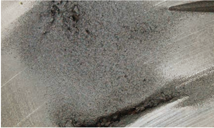
Figure 2. High viscosity can lead to cavitation and erosion caused by a collapsing air bubble or vacuum bubble.
