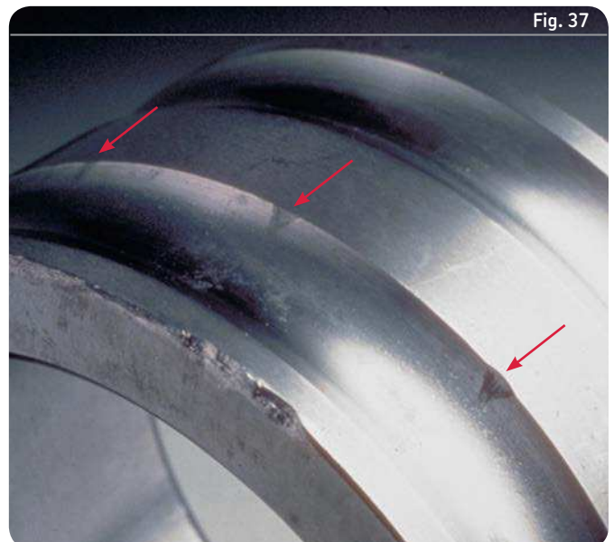
Indentations at ball pitch on the raceway of a double row angular contact ball bearing resulting from incorrect mounting
