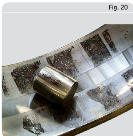
Corrosion on the outer ring and roller of a spherical roller bearing
