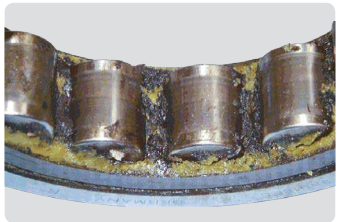
Cylindrical roller bearing outer ring with cage, rollers and grease Current leakage resulted in burnt grease (black) on the cage bars
