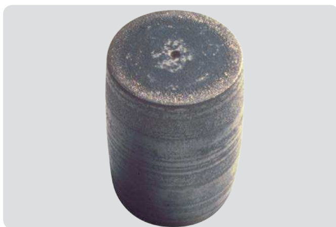
Spherical roller bearing – roller Corroded roller due to severe water penetration into the bearing
