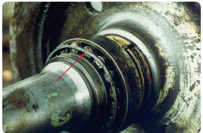
Tapered roller bearing mounted on a railway wheel set Cage was hit directly during mounting, resulting in permanent deformation (flattening)
