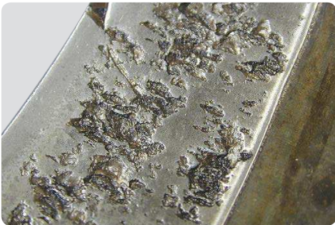
Spherical roller bearing outer ring Initially, abrasive wear due to contamination, developed into surface distress and advanced spalling
