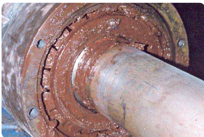
Tapered roller bearing in a pump unit Seal failure, bearing corrosion and reddish discolored grease
