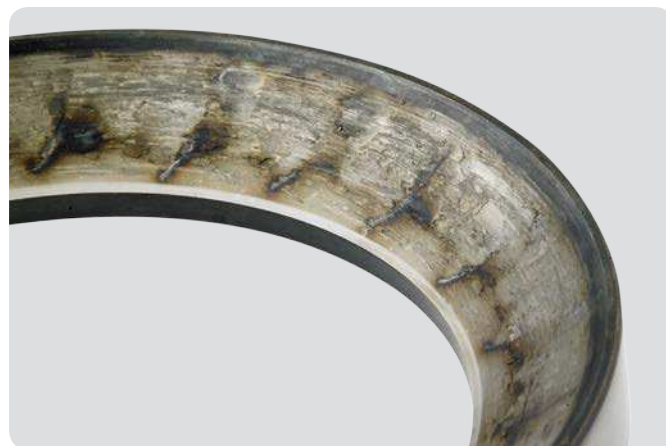
Spherical roller thrust bearing outer ring Initially adhesive wear, then excessive heat generation, finally jamming
