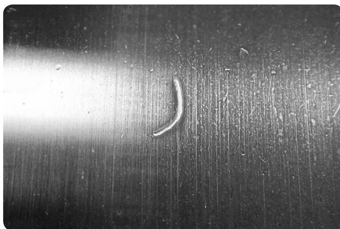
Spherical roller bearing outer ring Overrolled swarf/chip will lead to spalling
