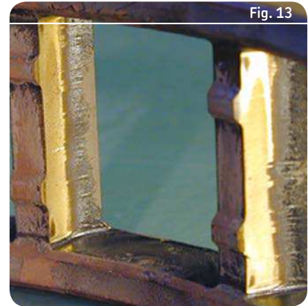
Abrasive wear on the cage bars of a cylindrical roller bearing
