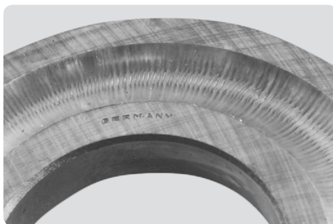
Thrust ball bearing shaft washer Exposure to vibrations at standstill, several sets of false brinelling marks at ball pitch
