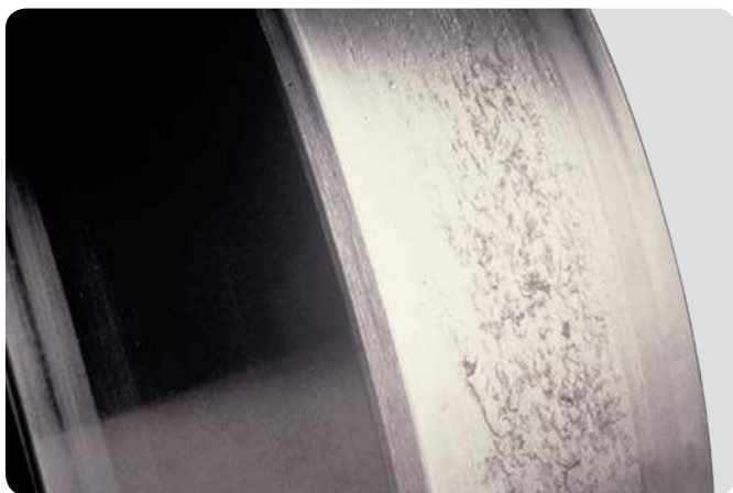
Spherical roller bearing inner ring Too low load combined with inadequate lubrication
