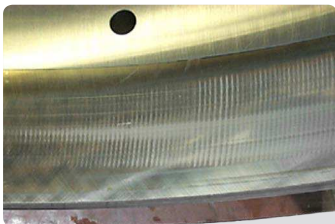
Spherical roller bearing outer ring Current leakage
