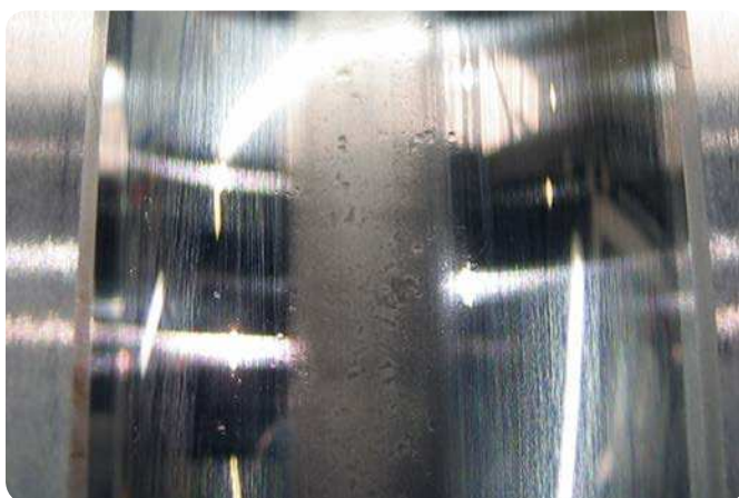
Deep groove ball bearing inner ring Dents resulting from overrolling of hard particles – inadequate sealing arrangement
