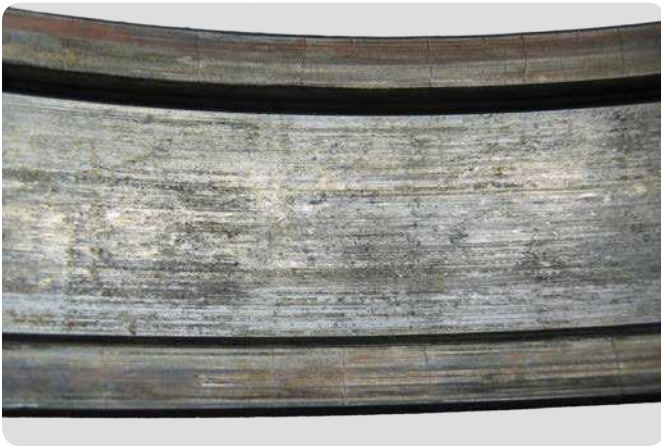
Cylindrical roller bearing outer ring Thermal cracks at both shoulder-cage contact due to inadequate lubrication
