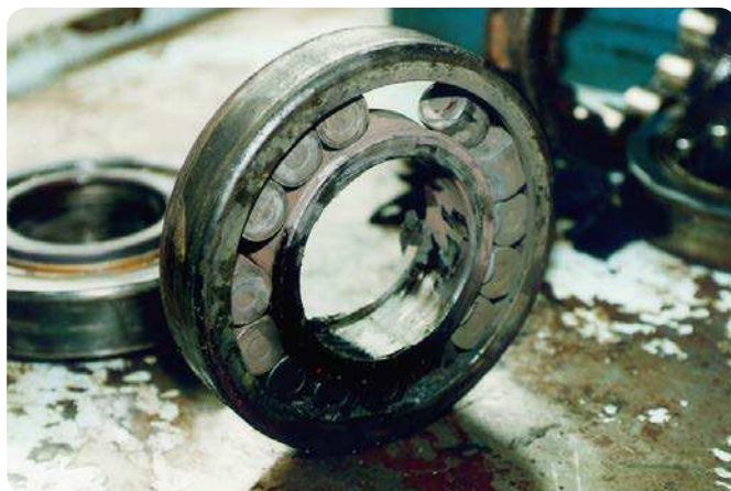
Cylindrical roller bearing – inner ring, outer ring and rollers Seized bearing – forced fracture of cage due to lubrication problem
