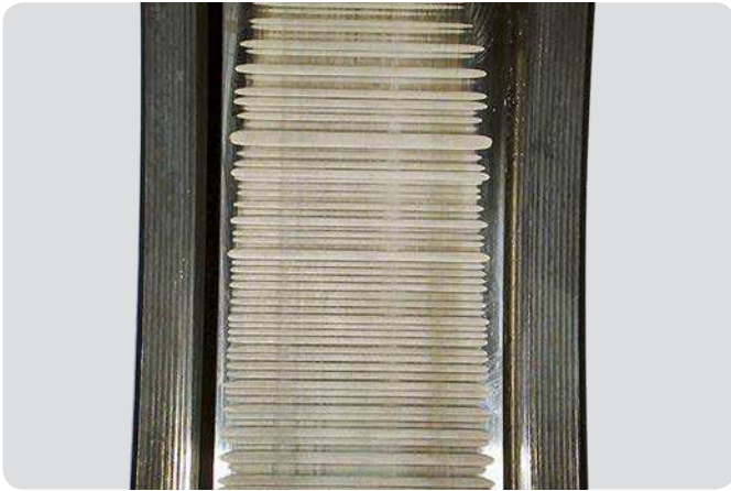
Cylindrical roller bearing outer ring Advanced stage of washboarding
