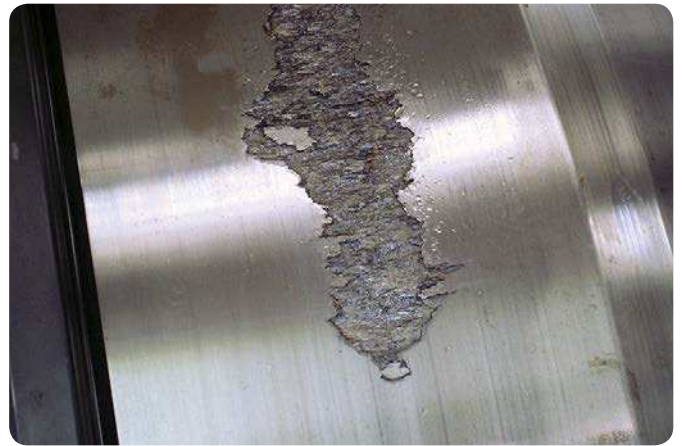
Spherical roller bearing inner ring Material fatigue
