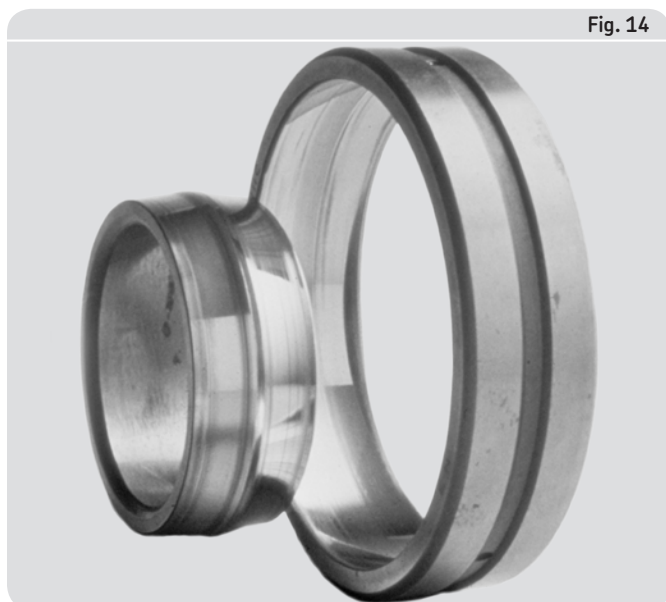
Polishing wear (mirror-like raceway surfaces) on the inner and outer rings of a spherical roller bearing
