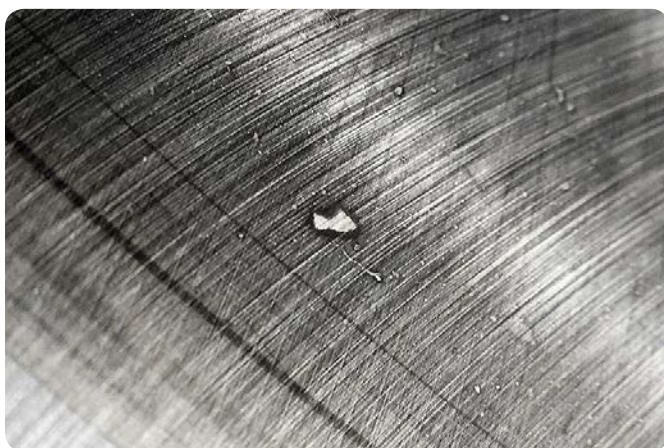
Spherical roller bearing outer ring Overrolling of hard particles that entered the bearing during mounting – lack of cleanliness
