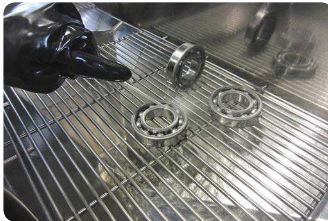
Cleanliness assessment (contamination analysis) – rinsing
