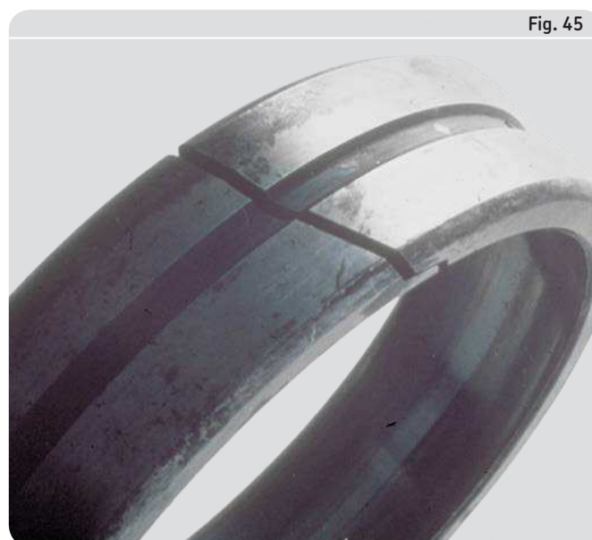
Fatigue fracture of an outer ring of a spherical roller bearing
